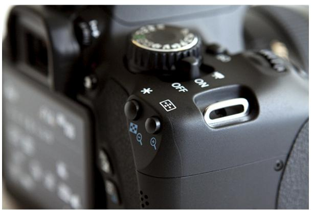
Figure 92 - Detail of the Canon T4i showing the AF Point Selection Button and the AE Lock Button [\*].
