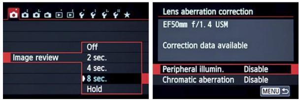
Figure 15 - Image Review menu (left), and Lens Aberration Correction menu (right) for the camera to automatically correct for lens issues when using Canon lenses, including Peripheral Illumination and Chromatic Aberration.
