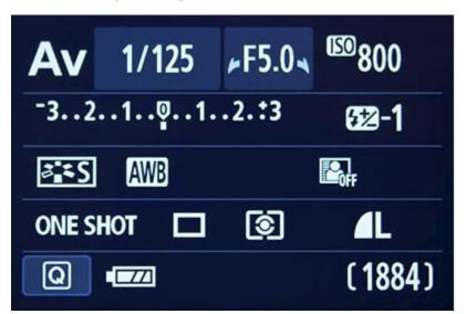
Figure 93 - Shutter Speed setting, Aperture setting, and ISO setting all shown on the top row of the Shooting Settings screen on the rear LCD Monitor. Because the camera is in Aperture Priority (Av) Mode, the arrows around the Aperture setting indicate you can turn the Main Dial to adjust this setting.
