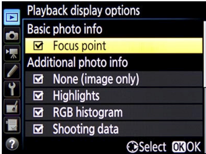
Figure 3.4 - Playback Display Options, allowing you to select which information and displays are available to view during image playback.
