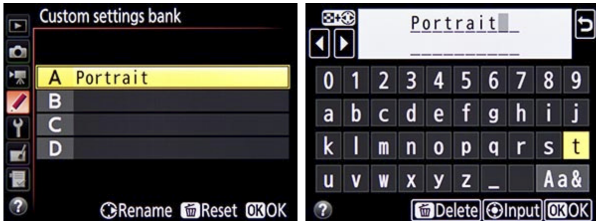
Figure 3.44 - The Custom Settings Bank (left), allowing you to register and save a group of selected settings. Press right on the Multi Selector to name the Bank, as shown at right.
