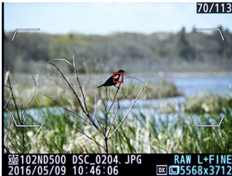
Figure 3.6 - File information view during image playback, with Focus Point Display enabled to show which Focus Point was used for autofocus with this shot, indicated by the tiny red square located on the bird, near the center of the frame.
