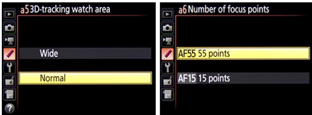
Figure 3.48 - 3D-Tracking Watch Area options of Wide and Normal. Right: Number of Focus Points, to choose if 55 AF Points or 15 AF Points are selectable in the Viewfinder.
