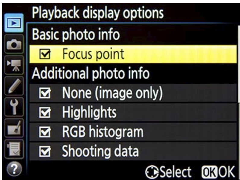
Figure 32 - Playback Display Options, allowing you to select which information and displays are available to view during image playback.
