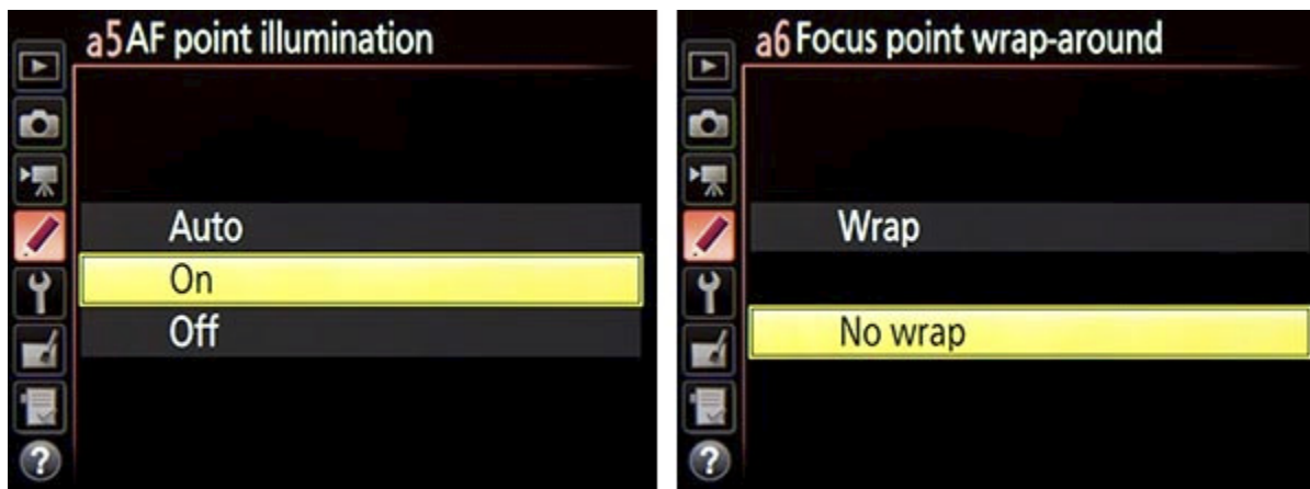
Figure 73 - Left: AF Point Illumination, to choose when the selected, active AF point will light-up in the Viewfinder. Right: Focus Point Wrap-Around, to choose if AF point selection stops at the edges or not.
