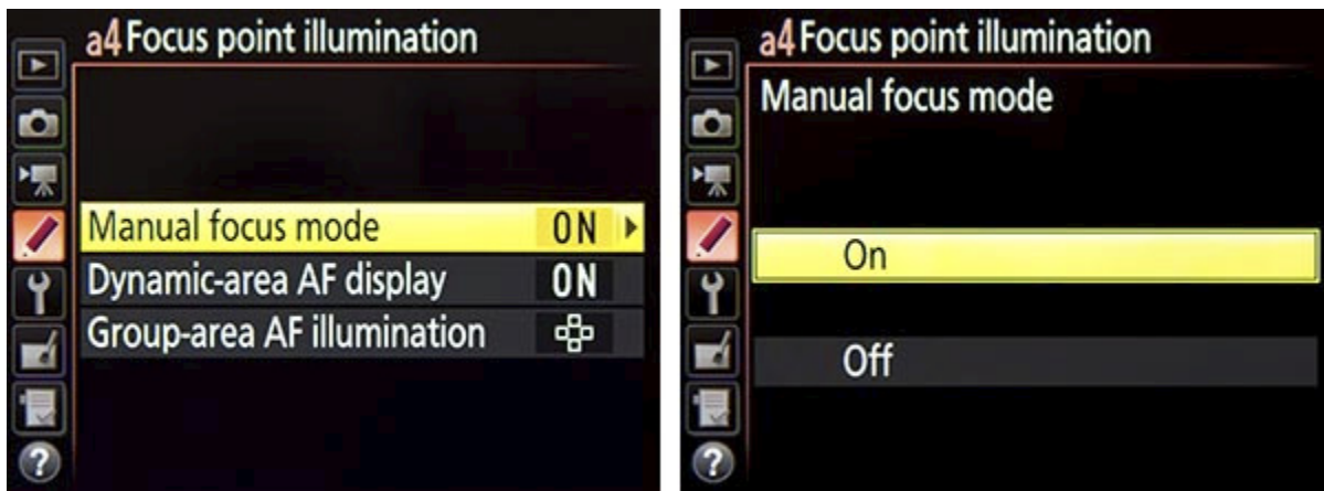
Figure 69 - Left: Focus Point Illumination options, to choose how the AF points are displayed in the Viewfinder, for various situations. Right: The Focus Point Illumination sub-menu options for Manual Focus Mode.
