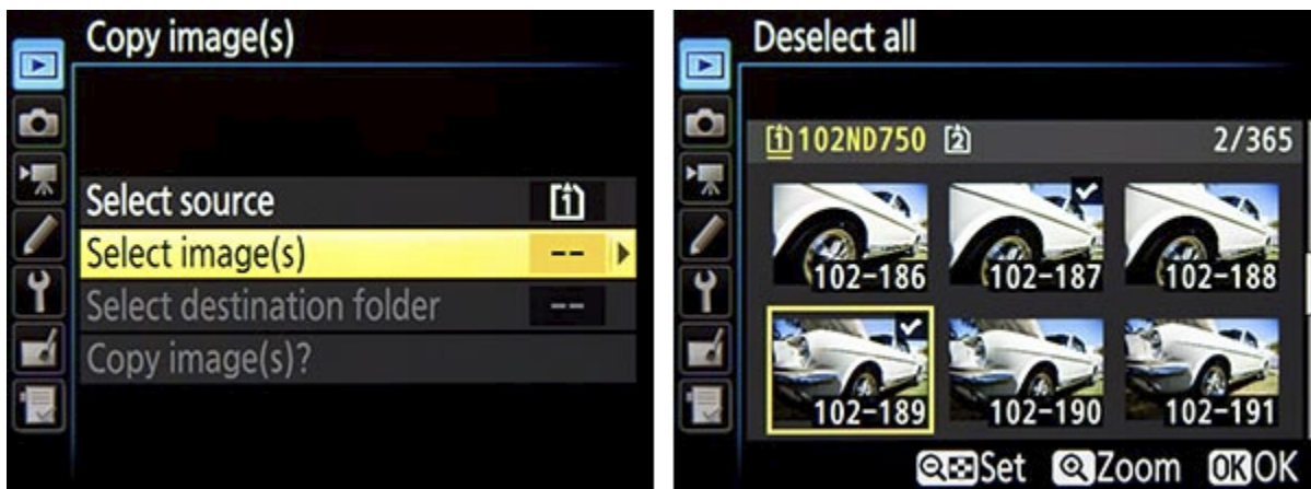
Figure 35 - Copy Image(s) Menu Item - Work your way down the options (left) to select the source card and the specific images (right). Then select the Destination Folder and choose “Copy image(s)” to complete.
