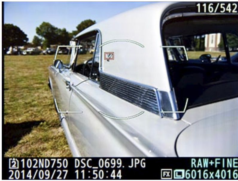
Figure 34 - File information view during image playback, with Focus point display enabled to show which Focus Point was used for autofocusing with this shot, indicated by the tiny red square located at the Thunderbird medallion on the side of the car.
