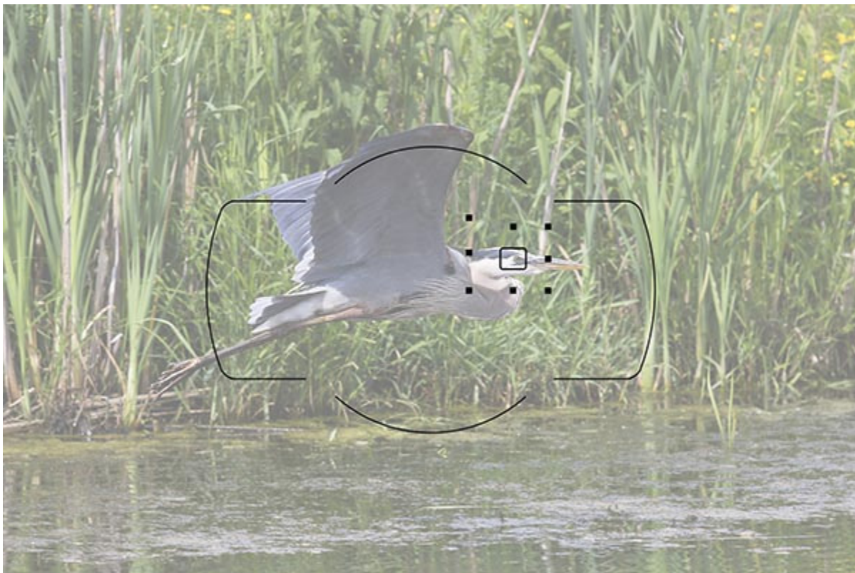
Figure 70 - Custom Setting a4: Focus Point Illumination - Simulated view of the D750 Viewfinder - Use the “Dynamic-Area AF Display” item of Custom Setting a4 to display just the single active AF point, or to display all of the points of the Dynamic-Area, as shown here with 9-Point Dynamic Area. Background image shown at 50% opacity to better see Viewfinder elements. Shutter speed 1/1600, Aperture f/4.0, ISO 200.
