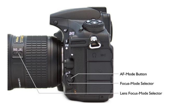
Figure 189 - Additional autofocus controls of the D810.
