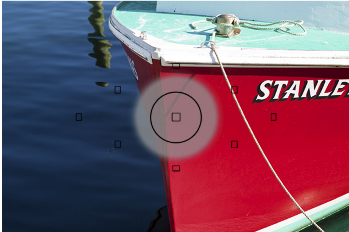
Figure 11 - Harbor, Gloucester, Mass. - Partial and Spot Metering Areas of the 60D - Partial Metering Mode evaluates only the area under the superimposed grey circle to determine the exposure settings. Spot Metering Mode evaluates only the area inside the black circle seen in the viewfinder to determine the exposure setting. Shutter speed 1/400, aperture f/4.0, ISO 100
